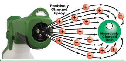
**Safer:** Electrostatic Wrapping: The E-Spray System's charged droplets reduces overspray and airborne mist.<sup>2</sup>
