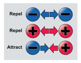
This concept is combined with the process of atomization. By applying an electrostatic charge to the liquid, each particle becomes charged with the same positive charge. Again using the basic principle that opposites attract and similar charges repel, the particles are naturally repelled by one another, and freely break apart or atomize. This is the primary concept that allows for a more even coating.
