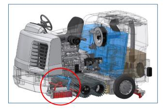
Figure 6: Passive heating of water from engine
