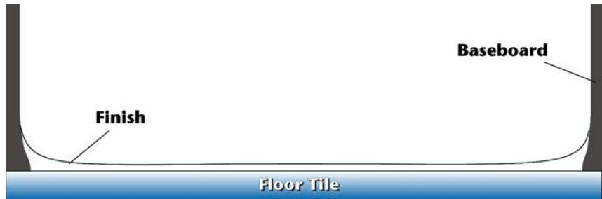
Illustration shows finish and build-up along walls and baseboards
